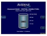
When the desired amount has been entered, pressing the "Fuel Done" button will exit the fuel initialization page.
