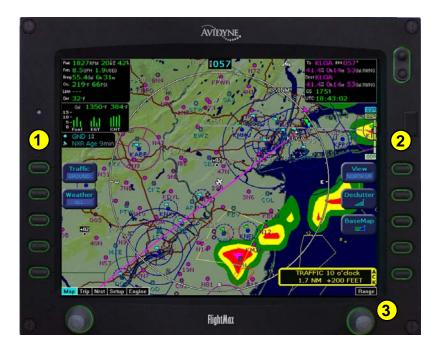
Sensor Functions - Control overlay and modes of available sensors. Buttons are only displayed for those sensors that are installed in the aircraft.
